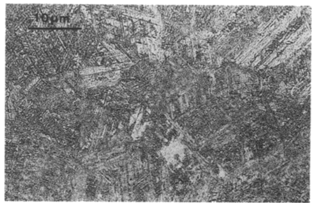
Figure 8 Optical micrograph of the alloy which transformed during mechanical testing, solution treated at 950° C for 1 h and air cooled.
